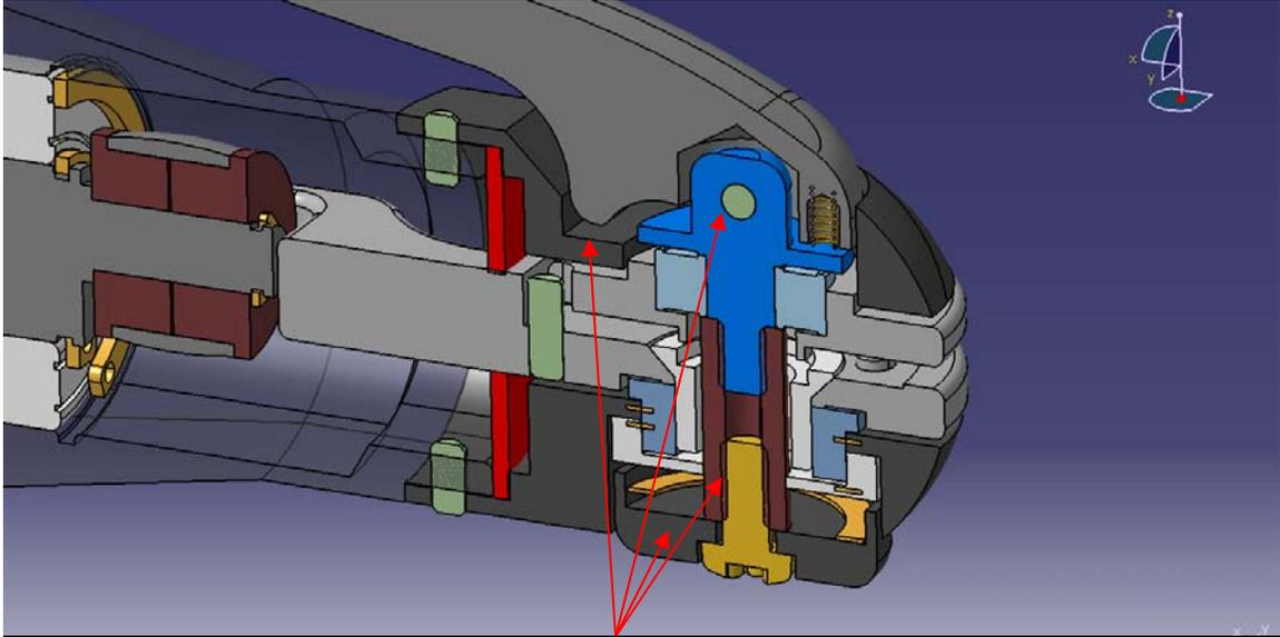
Bearing surfaces should be made out of a vacuum heat treated custom 455 stainless steel and should be coated with Medcoat 2000 to prevent any chances of corrosion.
